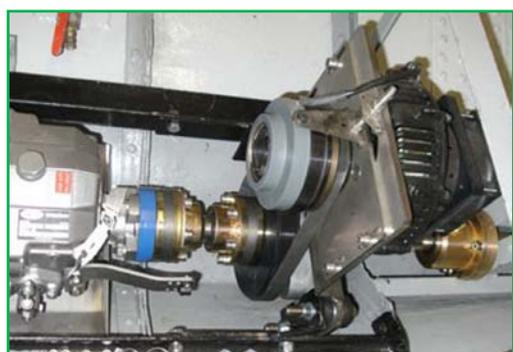
Standard delivery includes: PERM DC-Disc motor on adjustable support plate, mounting plate with pre-assembled thrust bearing unit, all installation materials (bolts, nuts etc.), electro-magnetic clutch, multi-belt and pulleys, all power cables (excl. cable from batteries to control box, pre-programmed control box with all necessary safety devices and fuses, switch panel, de-coupler for gearbox lever, control sensor-unit rev control.
