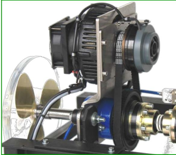
The **elsail Hybrid** is a so called parallel hybrid; the combustion engine ( diesel or petrol ) and the **elsail Hybrid** both drive the propeller, but not both at the same time.
